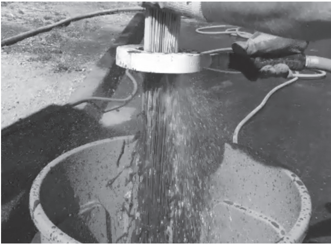
Rinsing Cartridge with Contech Rinse Tool
